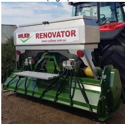
Figure 5. The Soil Kee renovator/ Planting system used in Australia to facilitate carbon sequestration
